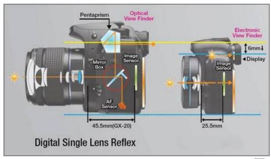
The light comes through the lens, reflects off the mirror, gets bounced around the pentaprism and is then seen via the viewfinder.
